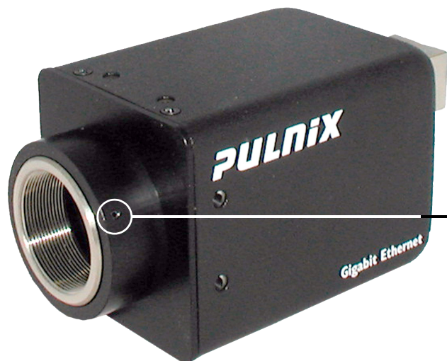
Figure 27. Back-Focus Set-Screw Locations
