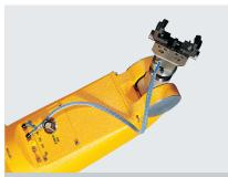
FOREARM CONNECTIONS Electrical and pneumatic connections close to the tool, user lines already installed.
