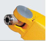
WRIST IP67 rating, submersible, high robustness, limited built-up on wrist.
