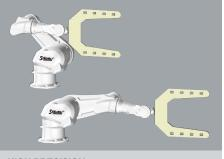
**HIGH PRECISION** High path precision on straight lines for slot loading/unloading
