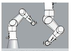
**MULTIPLE ATTACHMENT METHODS** Adaptability and flexibility (floor, ceiling).
