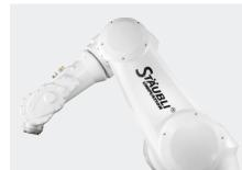
**ENVIRONMENT** The robot is available in different versions : Cleanroom, Humid Environment (HE), Food and Life Science applications.
