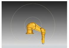
LARGE WORK ENVELOPE The short robot base enables it to work, shelf mounted on an injection molding machine for example.
