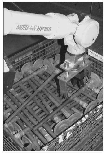
without regard to which side is up. The challenge was to decide the orientation and the location as well as the correct pick layer (Plate 4).
