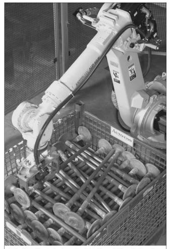
**Note:** Two-fingered gripper located at the middle activates when the axle is engaged to retain the axle for the move
