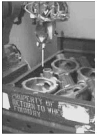
Plate 4 A Kawasaki robot picks vehicle brake rotors
