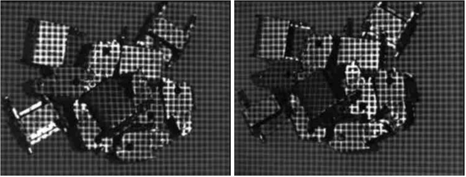
**Fig. 1.** An image pair showing a heap of unorganized parts with a high contrast grid projected on it.
