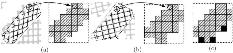
**Fig. 2.** Each intersection of a plane is represented as a pixel in the perspective invariant plane representation. Segmented plane from (a) left view, (b) right view. (c) Matching results for (a)-(b), intersection points with no correspondence are marked black.
