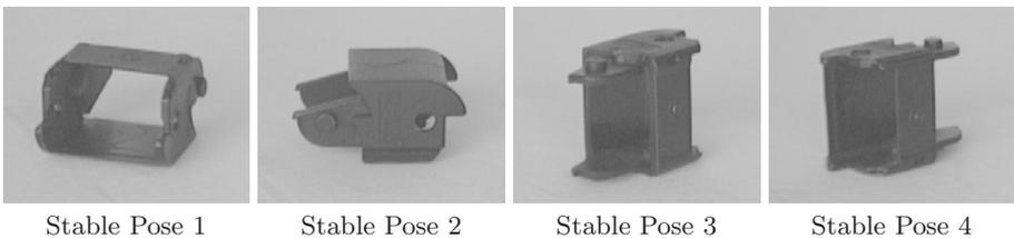
**Fig. 4.** Four stable poses of an industrial part.
