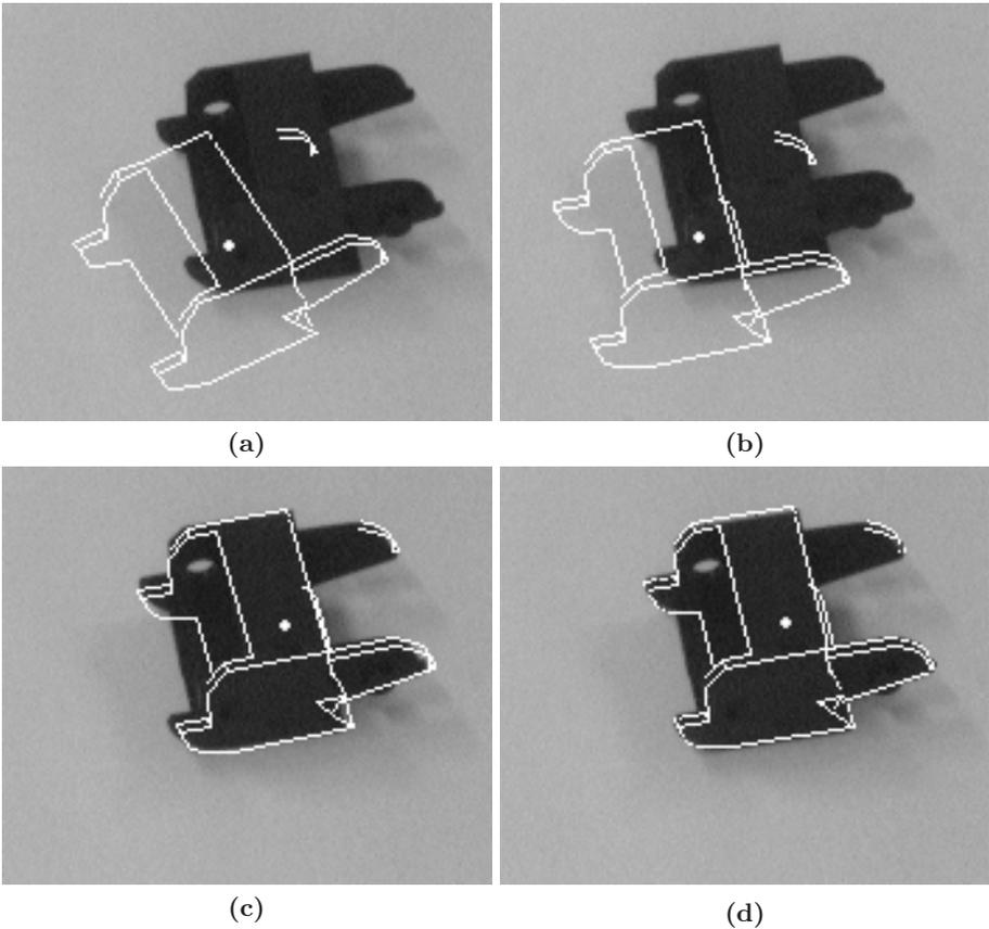
**Fig. 5.** The steps performed by the pose determination module visualized by superimposing the model projection on the image. The white dot indicates the center of gravity in 3D. **(a)** The CAD model placed on the center of the workplace, **(b)** rotation corrected, **(c)** rotation and translation corrected and **(d)** fitted. Note the difference on the left side of the object before **(c)** and after **(d)** the model fitting process.
