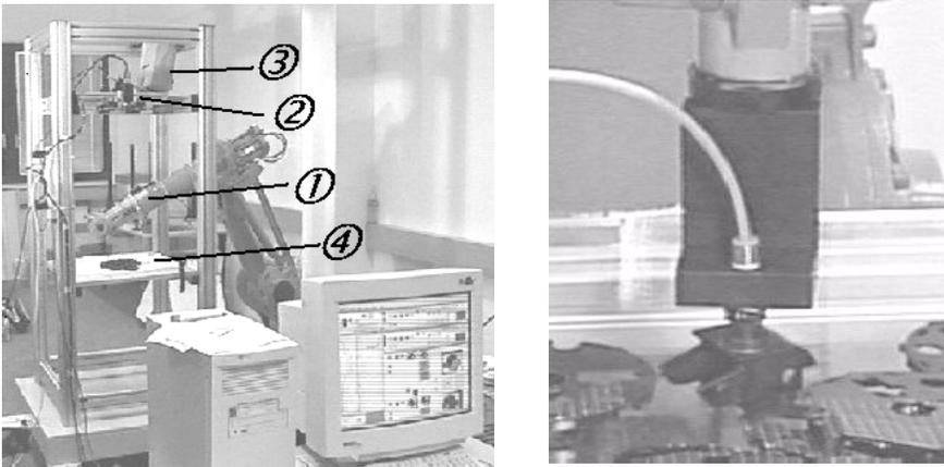
**Fig. 3.** (Left) The experimental setup consisting of a robot arm (1), a stereo rig (2), a grid projector (3) and a workplace (4). (Right) The robot picking a part from a heap of unorganized objects.
