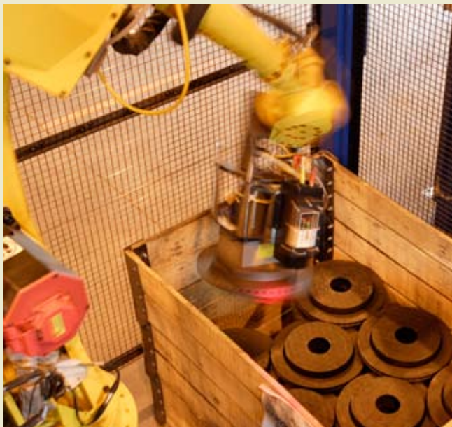
TRW's VGR solution is a semi-random bin-picking solution in which the robot searches for oriented parts within the bin. It was integrated by JMP Engineering
