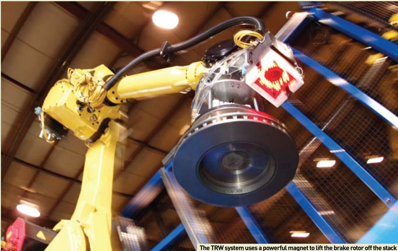
The TRW system uses a powerful magnet to lift the brake rotor off the stack
