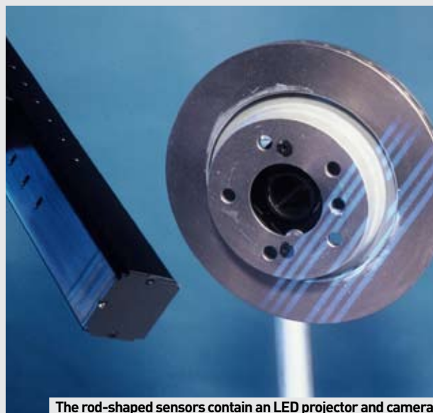
The rod-shaped sensors contain an LED projector and camera
