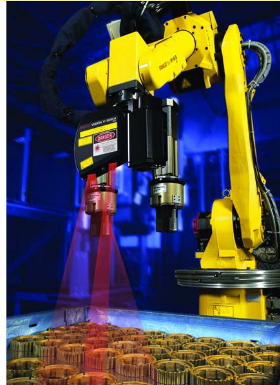
An Intelligent robot equipped with a FANUC vision sensor ideal for bin picking.
