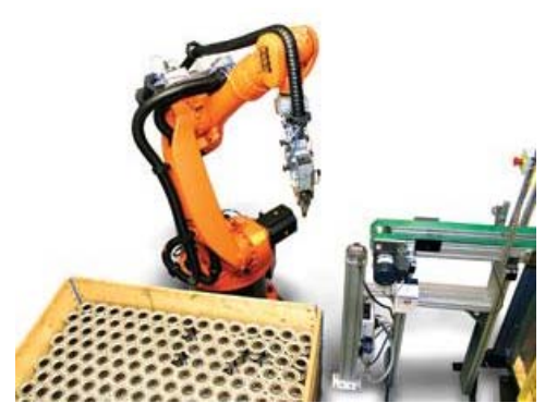
FIGURE 1. Rotorcan Workcell was developed by Scape Technologies for bin-picking applications at Grundfos. It can pick a rotor can part of a water pump from bin every 7.6 seconds, on average.
