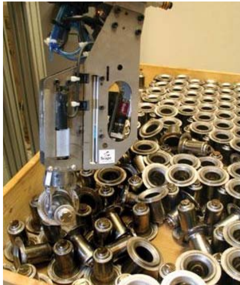
FIGURE 4. CAD files and a training program including a virtual camera were used to find the best features for geometric searches, as well as to determine the 15 standard gripping modes the robot uses. Click here to enlarge image
