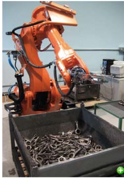
Random bin picking refers to a system where vision-enabled robots locate, grasp, and move single parts from a bin of jumbled or randomly piled parts.
