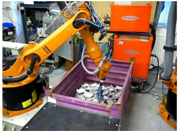
Figure 9 Experimental set-up for bin-picking of sheet-metal parts
