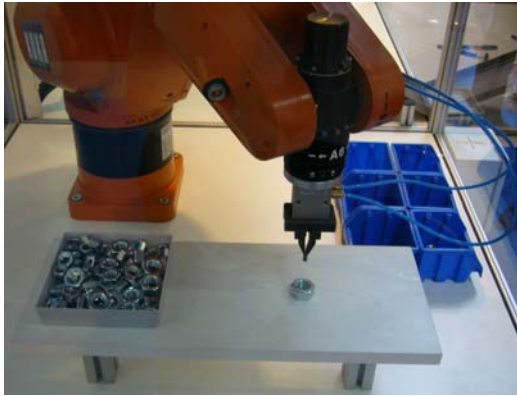
Figure 7 Experimental set-up for bin-picking of nuts
