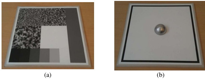
Fig. 3. (a) Front and (b) back of mobile test plate that has been created. Width is approximately 30 cm.
