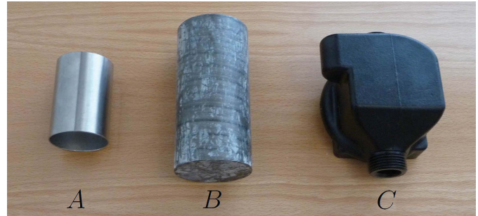
Fig. 1. Various objects with surfaces which may give problems when using 3-D scanners.
