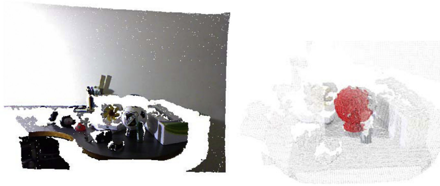
Fig. 1. Example of an original point cloud and object detection in the foveated cloud.
