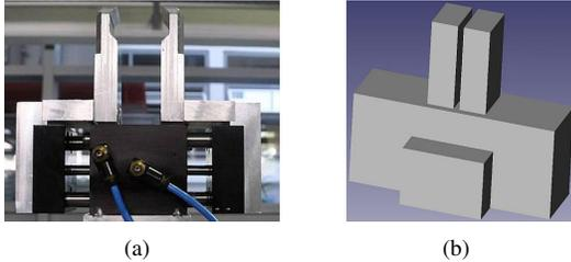
Fig. 4. The gripper used in the experiments. (a) Gripper. (b) CAD model.
