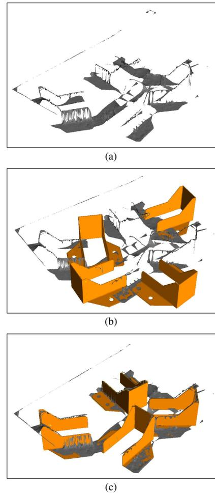
Fig. 3. Application of the RANSAM modification. Located Objects are displayed in orange, scan data in gray. (a) Scan of a bin filled with four joist hangers. (b) Erroneous localization result using the RANSAM with dipoles. (c) Correct localization result using the tripole variation.
