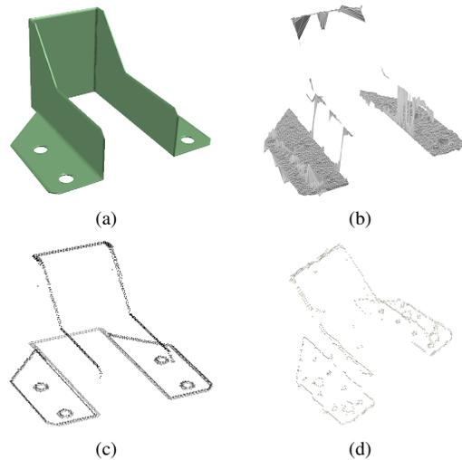
Fig. 2. Joist hanger. (a) CAD model, (b) scan from above, (c) CAD edge model, (d) scan edges.
