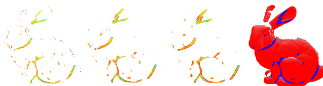
Fig. 2. From left to right: PFH persistence over multiple scales ( r_1 = 0.003 , r_2 = 0.004 , r_3 = 0.005 ) and the set of overall persistent points for the bunny00 dataset.
