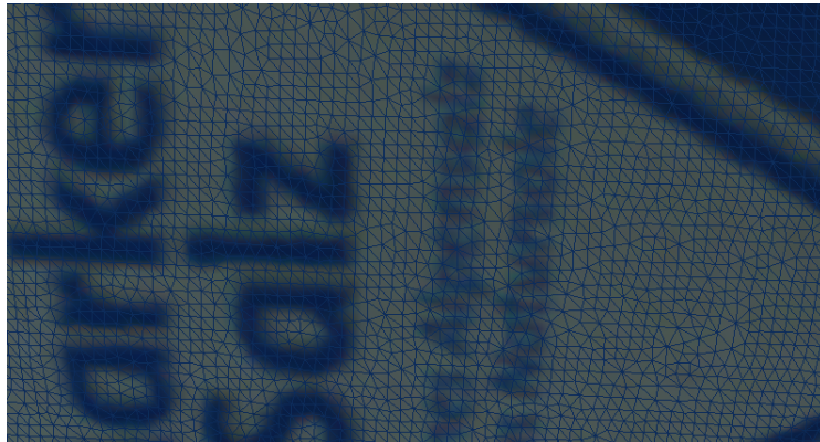
Figure A.1. A graphical example of the triangle meshes which a CAD model is made of with
