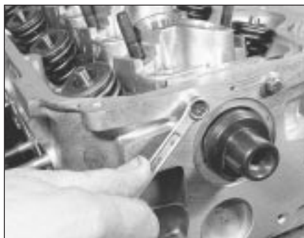
6.13a Unscrew the camshaft thrust plate bolts . . .
