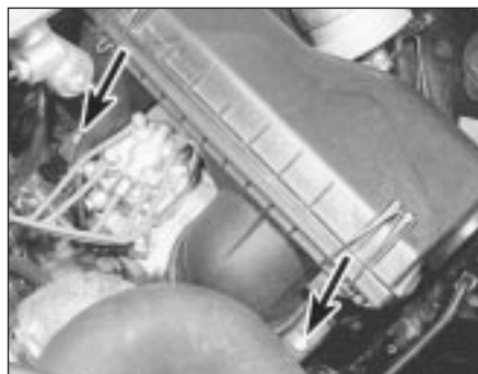
2.5 KE-Jetronic air cleaner retaining bolts (arrowed)
