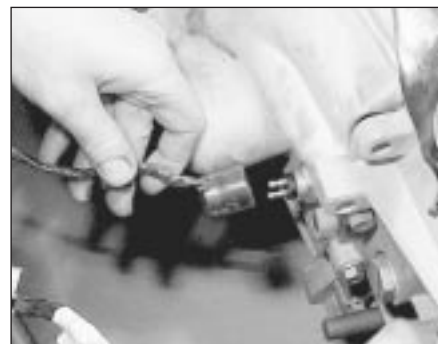
11.12e ... reversing lamp switch ...
