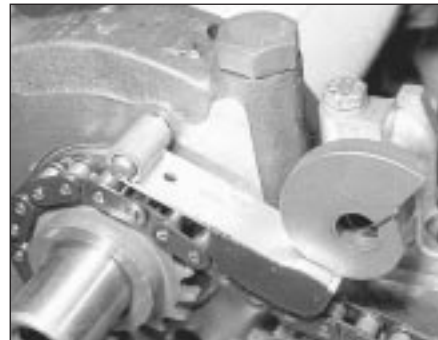
15.14 Refit the timing chain tensioner and arm
