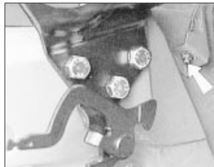
22.13 Cable tensioning block nut (arrowed) - Cabriolet models
