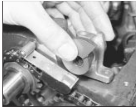
12.28 Removing the timing chain tensioner
