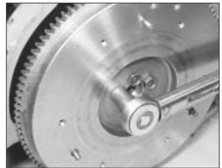
15.18b . . . then refit and secure the flywheel
