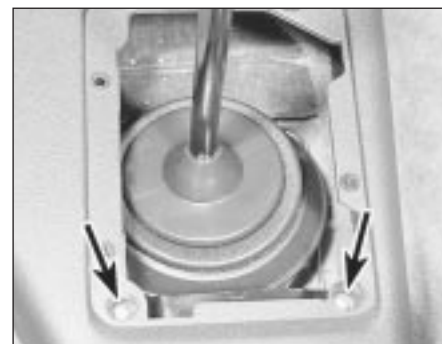
30.3a Centre console lower retaining screws (arrowed)
