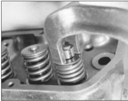
13.38 Compress the valve spring to remove the collets
