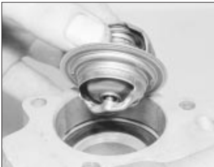
4.13b ... withdraw the thermostat ...
