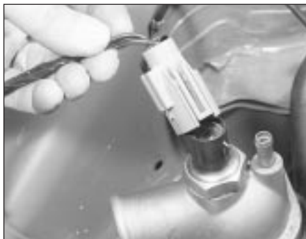
11.49a Disconnecting the cooling fan thermal switch . . .
