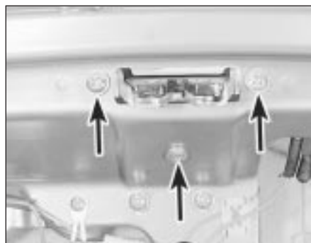
16.3 Tailgate lock retaining screws (arrowed)
