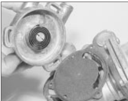
11.5 Removing the automatic choke bi-metal housing
