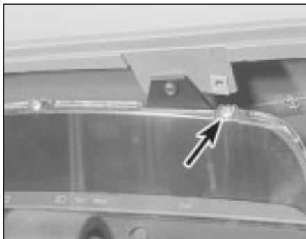
9.9a Instrument panel upper retaining screw (arrowed)
