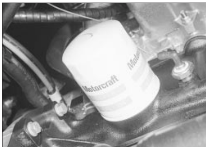
6.7 Oil filter location - CVH engine
