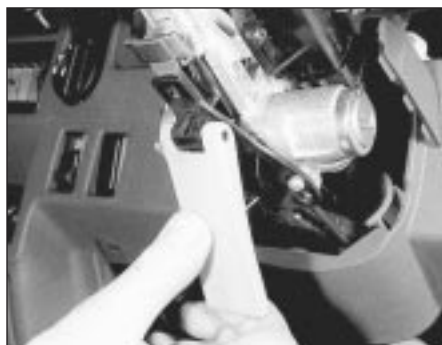
25.8 Removing the bonnet release lever
