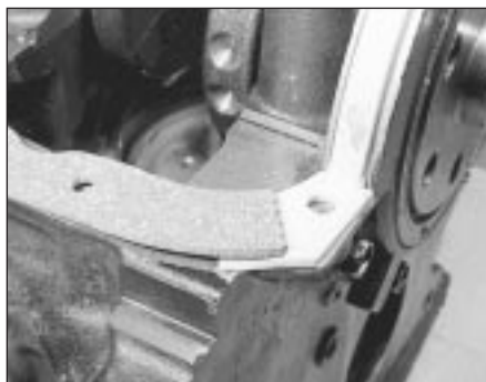
8.9b . . . followed by the side gaskets with their ends overlapped
