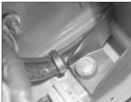
11.41a Radiator lower mounting bolt . . .
