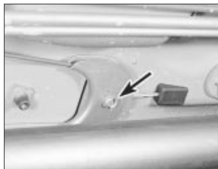
9.3b Primary cable-to-equaliser clevis pin and spring clip (arrowed)
