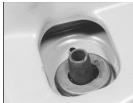
11.41b . . . and upper locating peg - HCS engine
