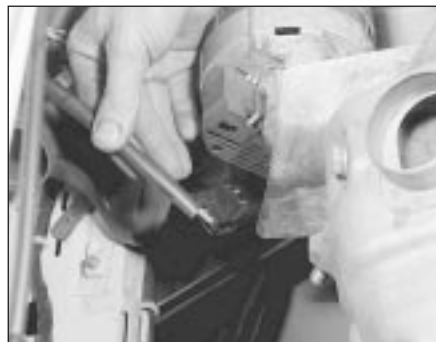
11.12a Disconnecting the alternator multi-plug ...
