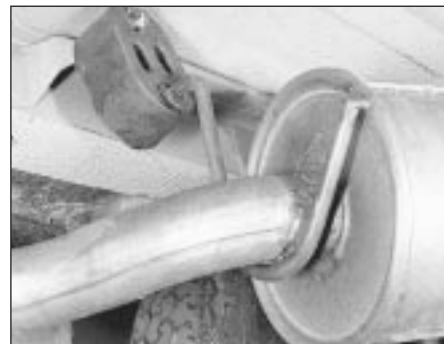
4.2b . . . and expansion box mounting
