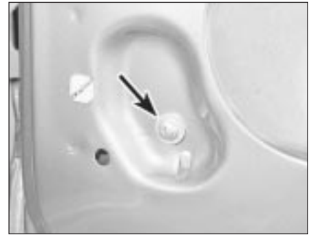
14.5 Glass run extension retaining screw (arrowed)
