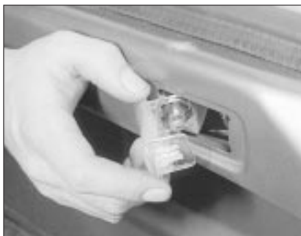
6.11 Removing the load space lamp
