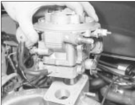
16.27 Lifting off the carburettor - 1.1 and 1.3 litre HCS engines
