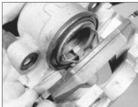
2.6 Removing the inboard pad from the piston housing . . .
