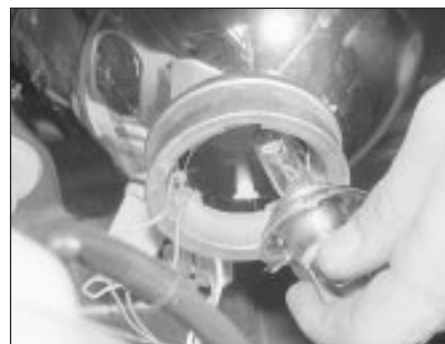
5.3 Headlamp bulb removal
