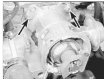
5.40 Distributor flange upper retaining bolts (arrowed) - CVH engines (electronic breakerless system)
