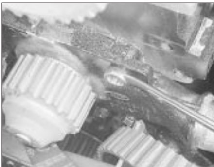
5.21a Undo the four bolts . . .
