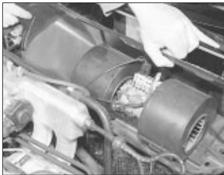
16.5b Removing the heater fan motor assembly . . .
