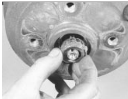
9.6 Rear hub outboard bearing removal
