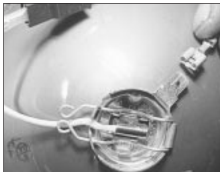
5.17 Disconnecting auxiliary lamp earth lead
