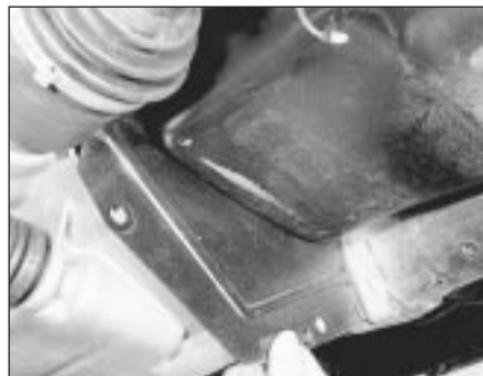
8.5 Remove the clutch housing cover plate
