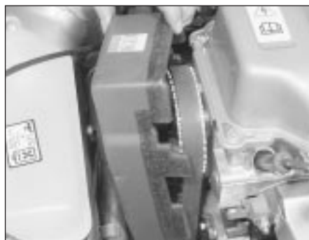
4.4b . . . and remove the upper half
