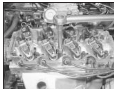
7.23b Tightening the cylinder head bolts
