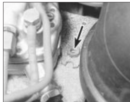
10.33 KE-Jetronic system mixture adjustment tamperproof plug (arrowed)
