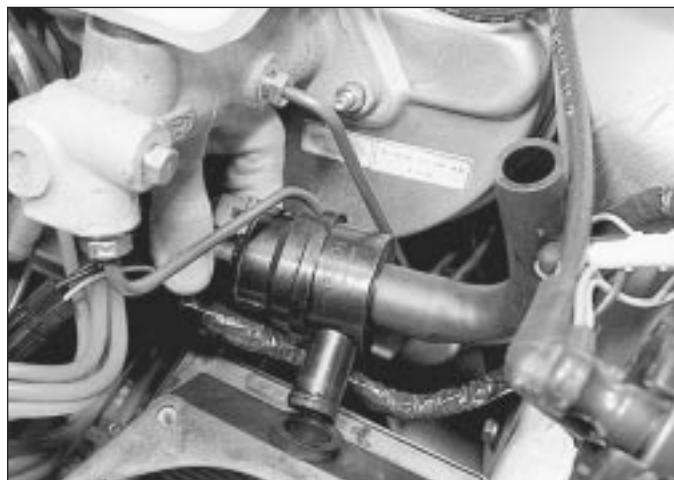
34.10b . . . withdraw the shut-off valve . . .
