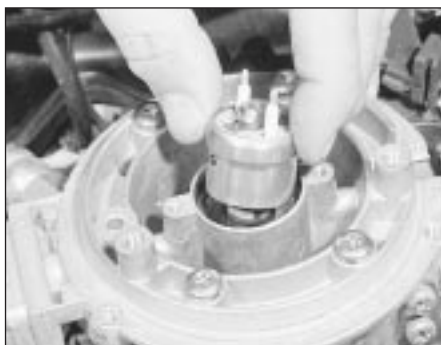
10.6 Withdrawing the injector from the CFI unit
