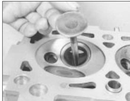
13.36 Inserting a valve into its guide
