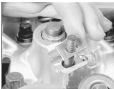
13.43a Fit the rocker arm spacer plate . . .
