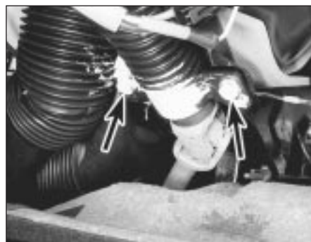
25.11a Steering column lower mounting clamp bolts (arrowed)
