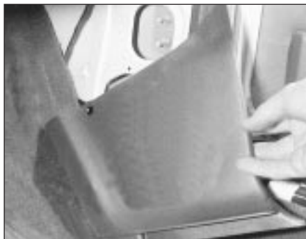
32.8 Removing cowl side trim panel
