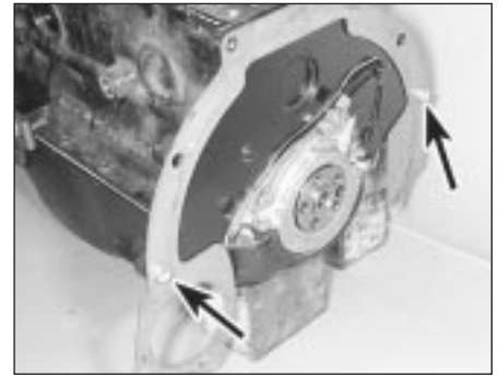
15.18a Locate the engine adapter plate over the dowels (arrowed) . . .
