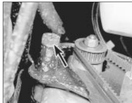
20.5 Modulator adjuster bolt (arrowed)
