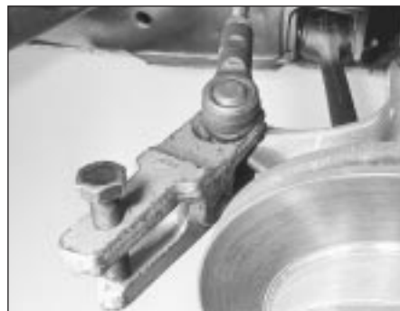
20.6 Releasing tie-rod balljoint using separator tool
