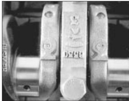
15.5b . . . with the arrows on the caps pointing toward the timing belt end
