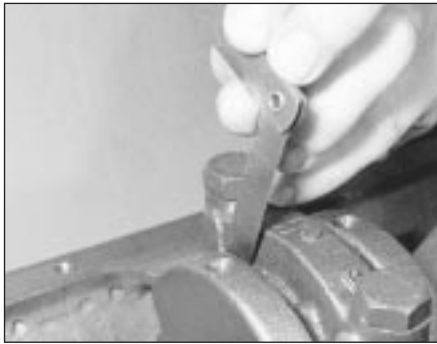
15.9 Using feeler blades to check crankshaft endfloat
