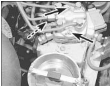
11.11 KE-Jetronic fuel distributor retaining screws (arrowed)
