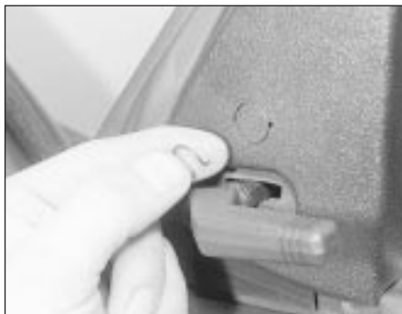
19.5a Remote control mirror handle circlip
