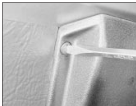
32.25 Releasing a tailgate moulded cover fastener
