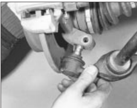
3.4b Separating the balljoint from the hub carrier
