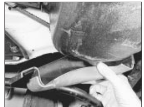
8.6 And the right-hand engine splash shield
