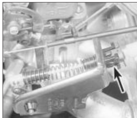
7.11b . . . then release the cable retainer (arrowed)
