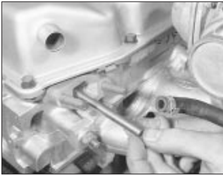
5.9 Removing the fuel pump push-rod
