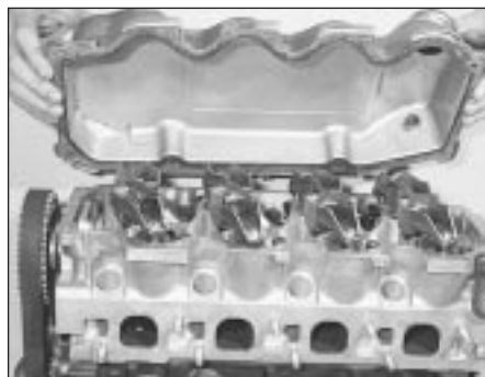
12.13 Remove the rocker cover
