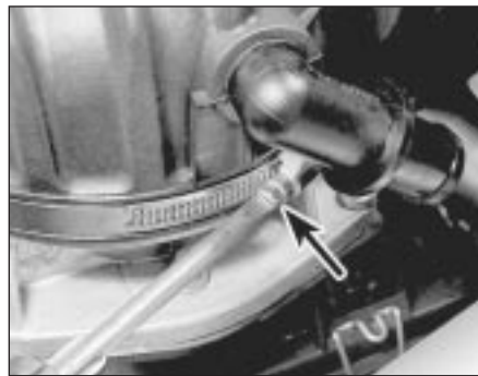
34.6a Slacken the securing band screw . . .
