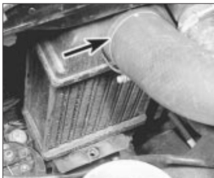
22.3 Intercooler upper air hose attachment (arrowed)
