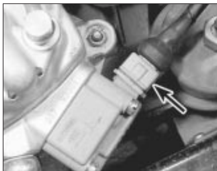
10.29 Pressure actuator wiring multi-plug (arrowed) - KE-Jetronic system
