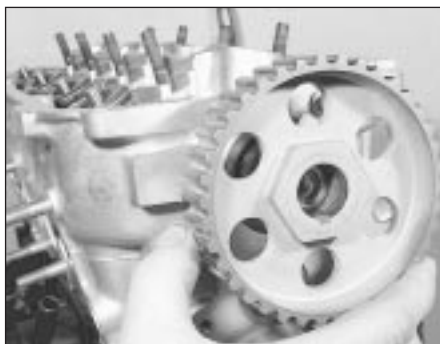
6.12 Removing the camshaft sprocket
