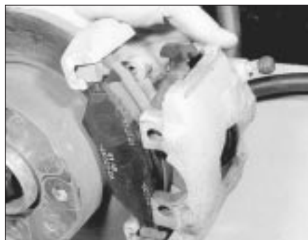
2.5 Withdraw the caliper piston housing
