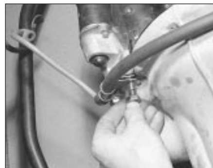
11.12h ... and starter motor connections on the 1.3 litre carburettor engine
