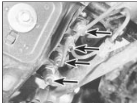
21.8 Hydraulic pipe and hose unions (arrowed) at the pipe bracket on the transmission support crossmember
