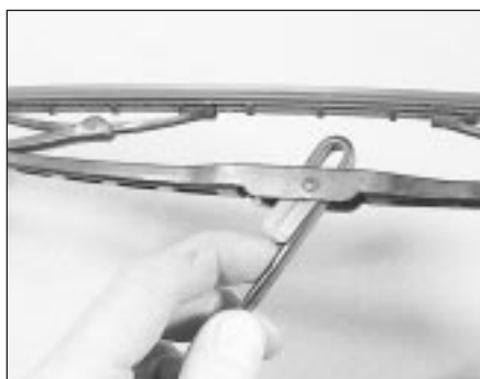
17.2 Disconnecting wiper blade from arm
