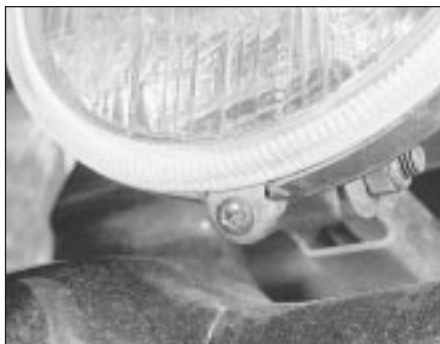
5.16 Front auxiliary lamp lens retaining screw
