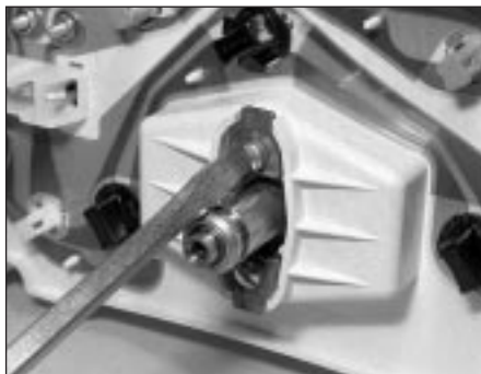
10.12a Extracting speedometer retaining screws
