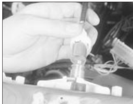
9.10 Disconnecting the speedometer cable
