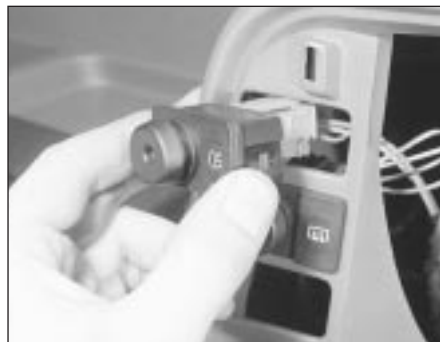
4.37 Rear foglamp switch removal - models from 1986 onwards
