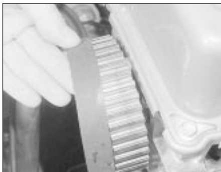
5.18 Removing the timing belt from the camshaft sprocket - CVH engine
