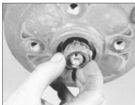
5.4 Remove the hub outer bearing . . .
