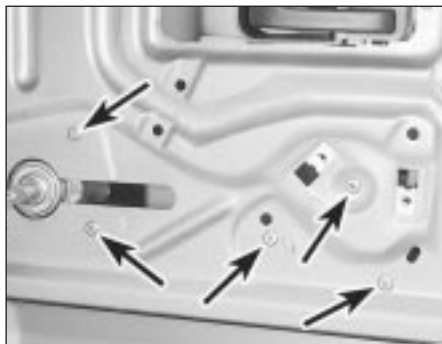
14.40b Regulator retaining rivet location (arrowed)
