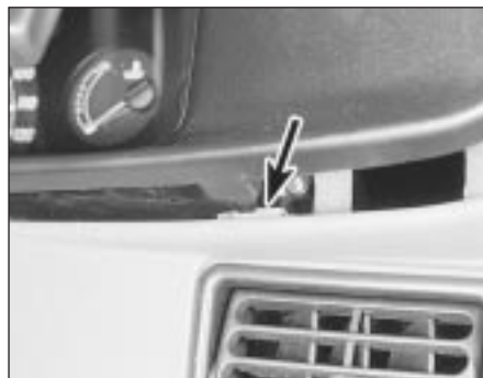
9.8 Bezel lower retaining clip (arrowed) - 1986 models onwards
