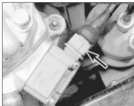
15.5 Pressure actuator wiring multi-plug (arrowed)
