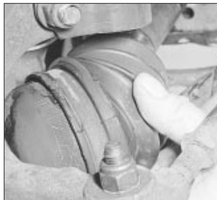
29.3 Checking driveshaft outer joint rubber bellows
