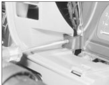
9.9b ... and lower screw removal - 1986 models onwards
