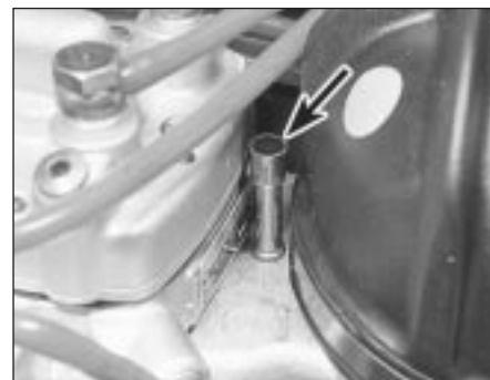
10.21 K-Jetronic system mixture adjustment screw location (arrowed)
