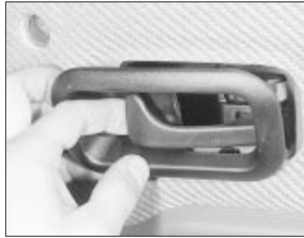
11.10b . . . and remove the bezel
