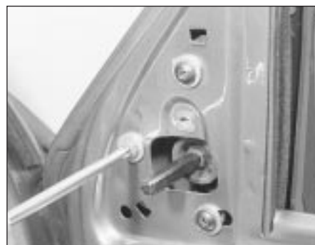
19.7 Removing the door mirror retaining screws
