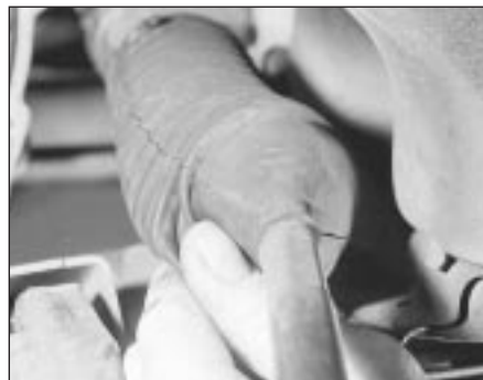
18.2 Checking a steering gear gaiter
