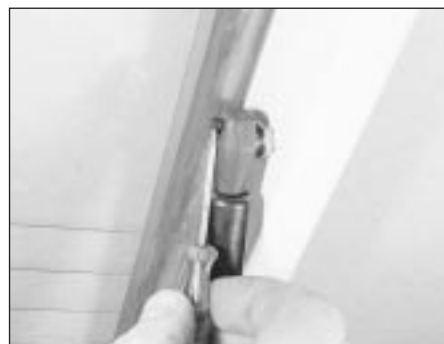
15.5 Releasing tailgate strut retaining clip
