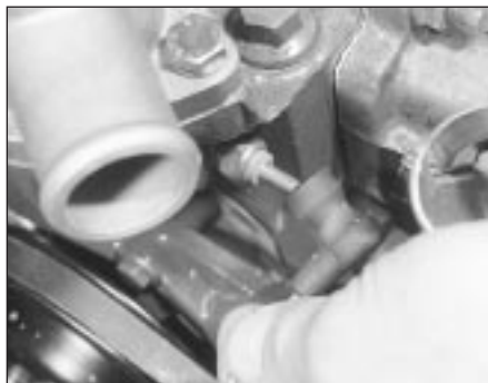
11.49b . . . and coolant temperature sender - HCS engine
