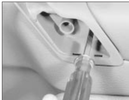
11.9b . . . undo the screws . . .
