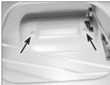
13.3 Door exterior handle retaining screws (arrowed)
