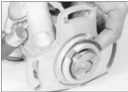
5.42 Checking the distributor O-ring seal condition - CVH engines (electronic breakerless system)
