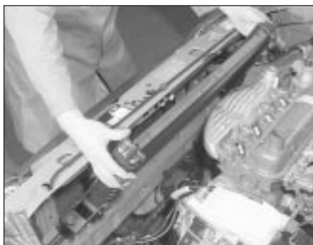
11.41c Lifting out the radiator - HCS engine
