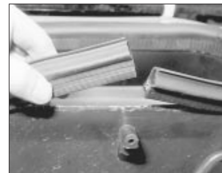
16.3 Remove the plenum chamber rubber seal
