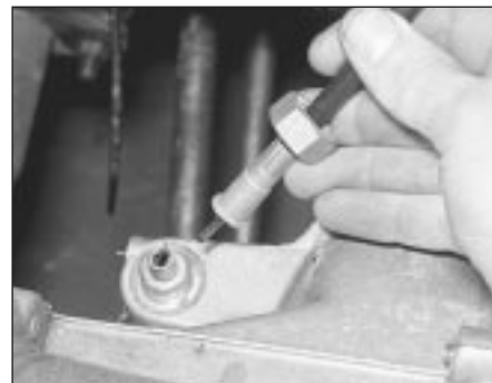
11.50 Disconnecting the speedometer cable - HCS engine
