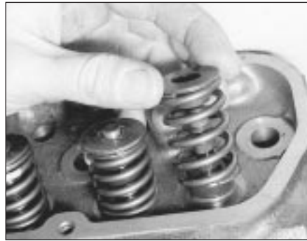
13.39 Remove the valve spring retainer and spring . . .
