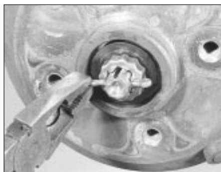
5.3b . . . extract the split pin and nut retainer . . .
