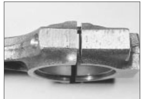
12.37 Connecting rod and big-end cap markings
