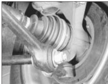
5.4 Anti-roll to lower arm retaining nut
