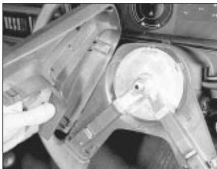
22.1a Steering wheel trim removal
