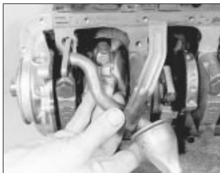
15.15 Fitting the oil pump pick-up tube
