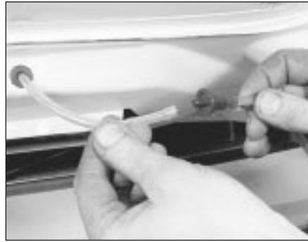
7.2 Disconnecting the windscreen washer fluid pipe
