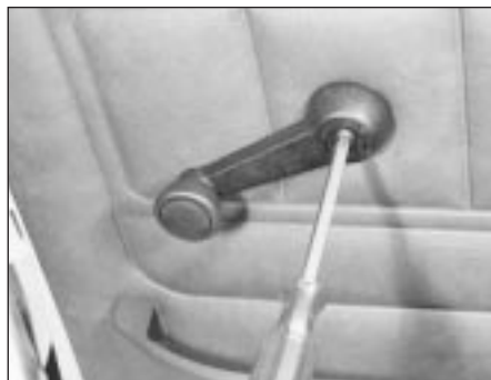
11.2b . . . and unscrew the regulator handle
