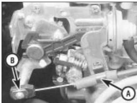
9.17b Choke cable outer cable clamp (A) and end fitting (B) on 1.3 litre HCS engine
