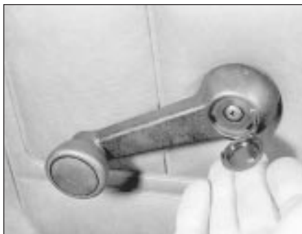
11.2a Prise out the plastic insert . . .
