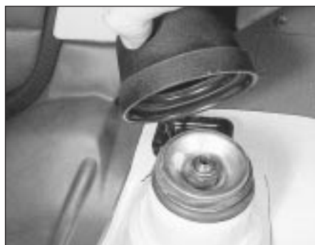
10.3 Rear shock absorber top mounting
