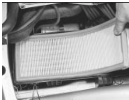
34.10d . . . and withdraw the element - K-Jetronic system
