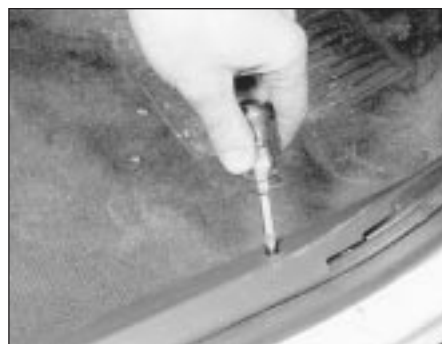
32.7 Removing a sill scuff plate securing screw
