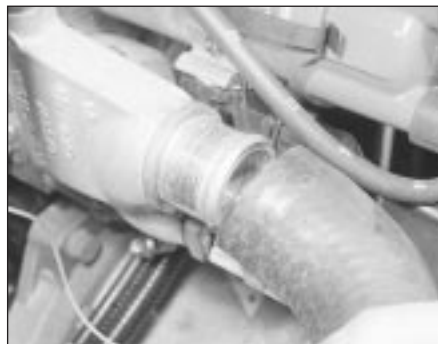
7.4 Disconnecting the hose from the thermostat housing - carburettor engine
