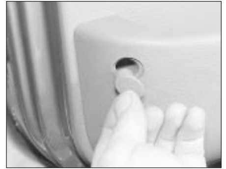
11.11a Release the trim cap and undo the screw . . .
