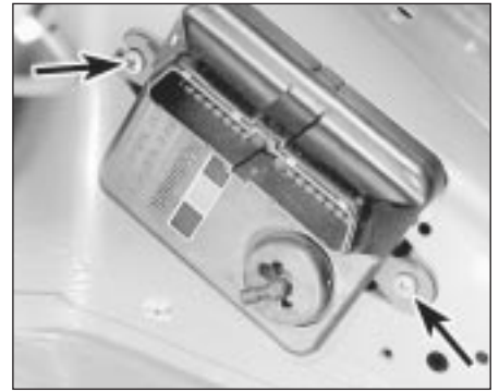
6.19 ESC module securing screws (arrowed)
