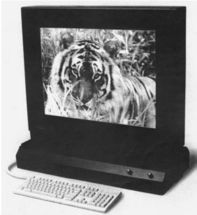
FIGURE 93.4 The 40-in. diagonal ac driven plasma display from Photonics Imaging. (From Friedman, P.S., Inf. Display , 11(10), October 1995. With permission.)
