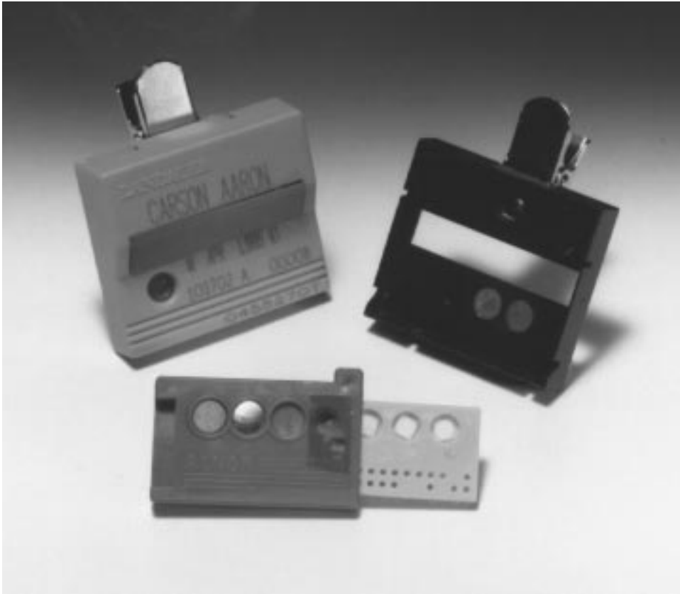
FIGURE 69.2 Thermoluminescence dosimeter body badge. A standard TLD badge contains three LiF phosphor chips. A fourth chip and a fast neutron track-etch foil can be added if required. (Courtesy of Landauer, Inc.)
