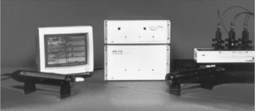
FIGURE 29.28 Three-component LDV system with fiber-optic probes.
