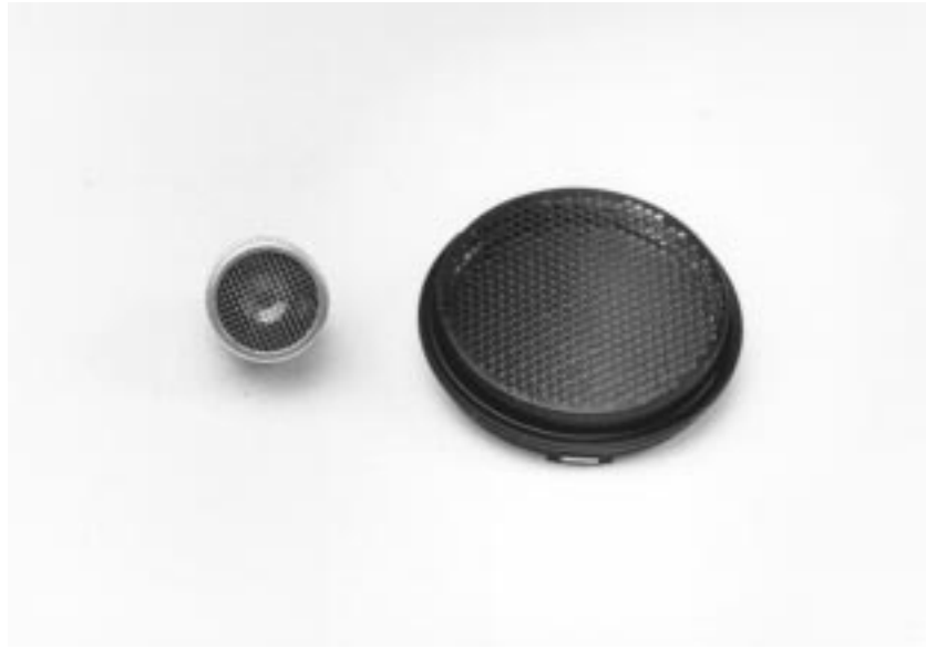
FIGURE 6.64 Ultrasonic transducers piezoelectric (left) and electrostatic (right).
