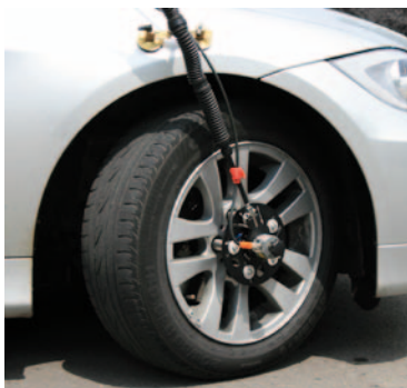
Fig. 2: WPT sensor mounted at the front wheel
