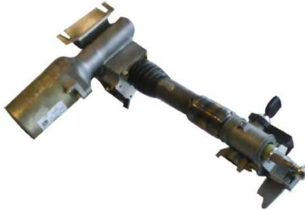
Figure 1.5: AtlasCar electrically controlled steering column.
