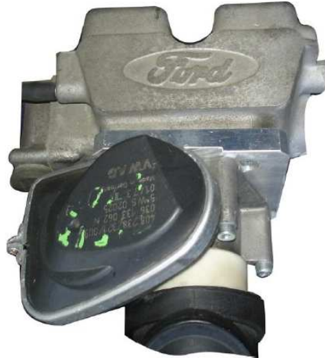
Figure 1.3: AtlasCar electronic throttle valve.
