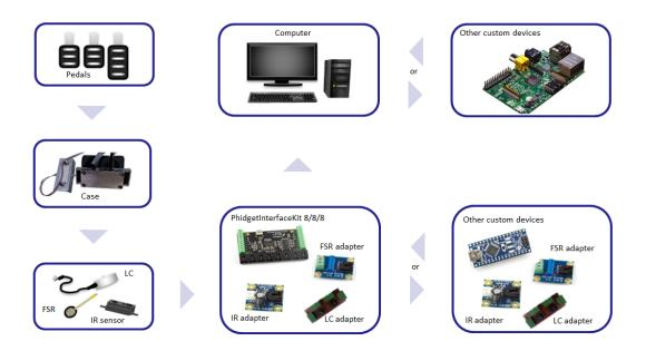
Figure 2.14: Setup scheme. In order to monitor the pedals, the case is mounted on them. The case has LCs,FSRs and IR sensors installed and these are connected to their adapters. The adapters connect to the PhidgetInterfacekit and than to the computer. It is possible to replace these adapters and the PhidgetInterfacekit for other custom devices. Also, it is possible to replace the computer for other device, such as a single board computer (SBC).
