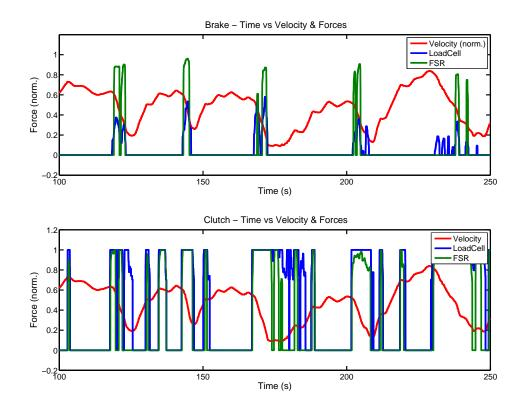
Figure 4.4: Data of the preliminary test from brake (top) and clutch (bottom) pedals, with a median filter applied, between 100s and 250s.
