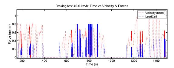
Figure 4.13: Data analysis for 40 km/h using only the brake pedal to stop the car. Only the periods where there were relevant braking forces are shown, the dotted lines represent the excluded braking periods.
