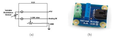
Figure 2.9: a) Force Load Cell adapter circuit scheme. b) Force Sensitive Resistor Adapter [20].
