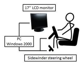
Figure 1.3: Driving simulator to collect behaviour signals [10].
