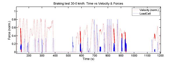
Figure 4.14: Data analysis for 30 km/h using only the brake pedal to stop the car. Only the periods where there were relevant braking forces are shown, the dotted lines represent the excluded braking periods.
