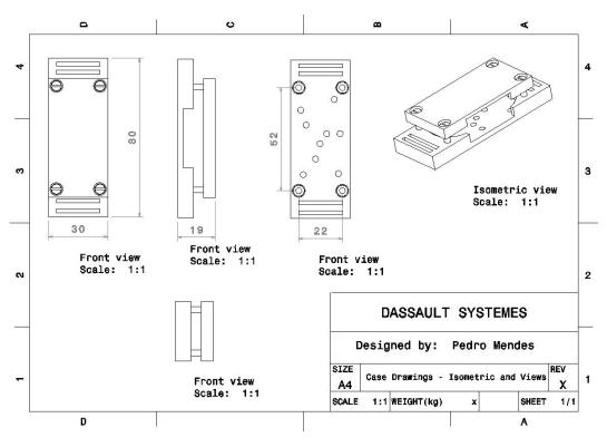
Figure 2.5: Case mechanical drawings.
