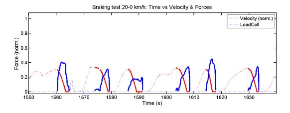
Figure 4.15: Data analysis for 20 km/h using only the brake pedal to stop the car. Only the periods where there were relevant braking forces are shown, the dotted lines represent the excluded braking periods.
