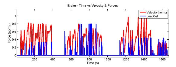
Figure 4.10: Data collected for different velocities using only the brake pedal to stop the car.
