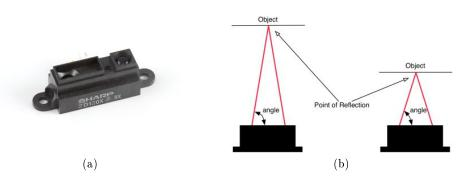
Figure 2.3: a) Sharp Distance IR Sensor (4-30cm) [17]. b) Sharp IR detector angle of reflection arrival for near and far object [17].
