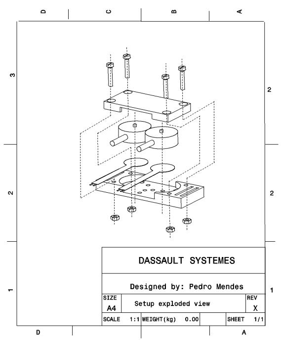
Figure 2.8: Exploded view of the case.
