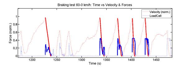
Figure 4.11: Data analysis for 60 km/h using only the brake pedal to stop the car. Only the periods where there were relevant braking forces are shown, the dotted lines represent the excluded braking periods.
