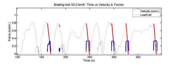
Figure 4.12: Data analysis for 50 km/h using only the brake pedal to stop the car. Only the periods where there were relevant braking forces are shown, the dotted lines represent the excluded braking periods.
