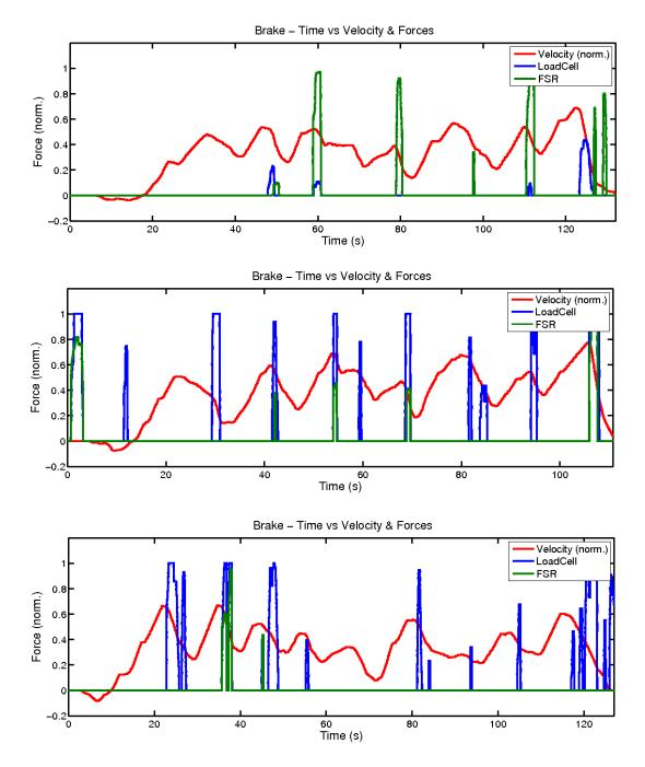
Figure 4.6: Data collected in the first test, for the same route, same car and different drivers. Top: Subject A; Middle: Subject B; Bottom: Subject C.
