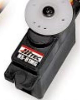
44.334 HS-81 25€ 44.336 HS-81MG 34€ - 16,6g (MG : 19g) - MG : pignons métal - 30x12x30mm - 3,0 kg.cm, 0,08sec/60°
