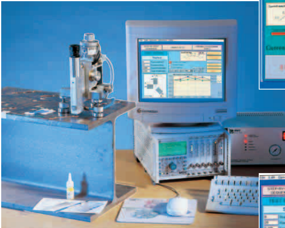
Complete measuring chain with amplifier and control PC
