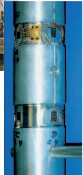
Dynamometer on a Sailing boat made by Technical University of Berlin with HBM strain gages (series Y)
