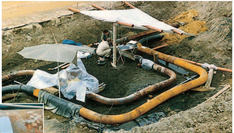
Strain gage application for stress analysis on pipes
