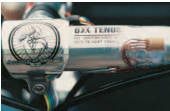
Strength testing of new type materials for high quality sports bicycle
