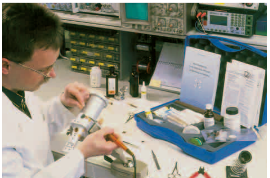
Special transducers which are constructed, applied and tested in the strain gage application laboratory.
