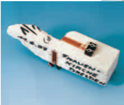
Stress investigation on a building material sample, using strain gages
