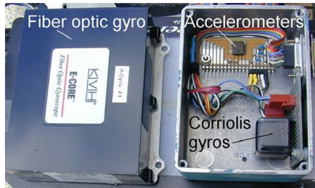
Figure 3: The inertial components of the attitude measuring system: KVH fiber-optics gyroscope, Gyration two-axes Coriolis gyroscope and an Analog Devices two-axis accelerometer.
