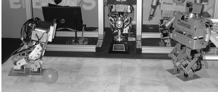
Fig. 3. Humanoid robots Robo-Erectus RE40I and RE40II (RE40I acts as a kicker while RE40II performs as a goal-keeper)
