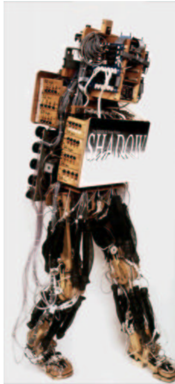
Figure 2.1: A photograph of the Shadow biped robot. Note the use of pneumatic 'air' muscles. (Source http://www.shadow.org.uk/ )
