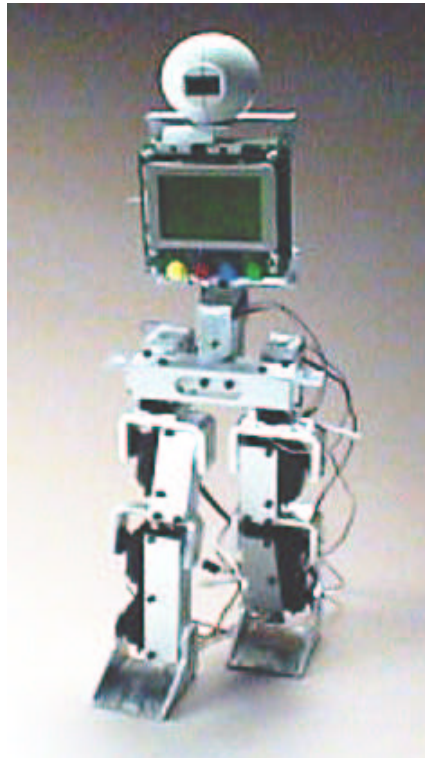
Figure 3.5: A photograph of the constructed robot. Overall the robot characteristics were as planned except for the COM. However the balance was found to be exceptional, with the robot being able to statically balance quite stably without actuation in an upright position.
