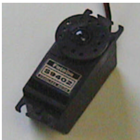
Figure 3.2: A photograph and specifications of the Futaba S9402 servo.
