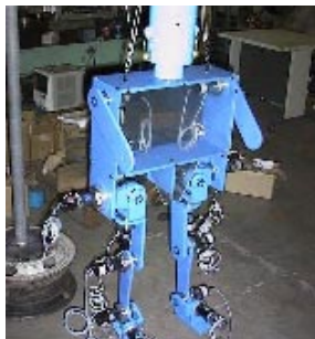
FIGURE 10. Biped under construction for investigation of the proposed control algorithms. From: http://www.kawalab.dnj.ynu.ac.jp/~fujimoto/biped.html
