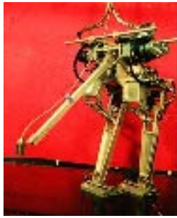
FIGURE 4. Meltran II, a six DOF biped with an ultrasonic sensor to measure the height of the floor 30 cm ahead of the hip joint. From Kajita: http://robby.caltech.edu/~kajita/biped.html
