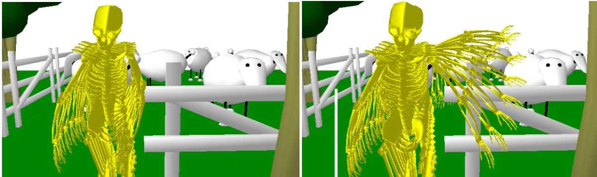
Figure 12: By rerunning the warping module only, different solutions are explored as the collision free motion is randomly searched. On the left image, the arm goes in front of Eugene, while on the right image the arm goes over the barrier.
