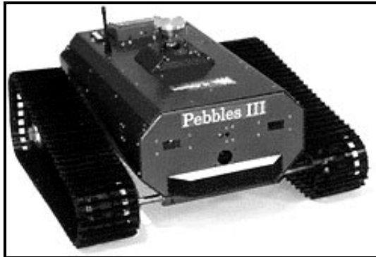
FIGURE 4. Pebble, a small tracked mobile robot by IS Robotics Ltd. [ISR].
