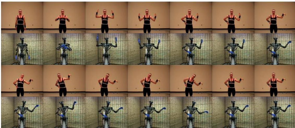
Figure 1: The Sarcos humanoid robot at ATR (DB) tracking motion capture data of a human actor
