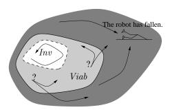
Figure 3: The viability kernel (Viab) is the set of all the states from where it is possible to avoid to fall. For a given control law, a fall is avoided only in an invariant set (Inv), a sub-set of the viability kernel.
