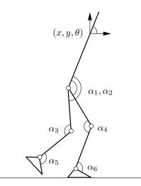
Figure 1: The configuration of a 6-DOF planar biped robot can be expressed through 9 variables, 3 for the global position of the robot  $(x, y, \theta)$  and 6 for its internal shape  $(\alpha_1, \ldots, \alpha_6)$ , to obtain the state vector  $q = (x, y, \theta, \alpha_1, \ldots, \alpha_6)^T$ .
