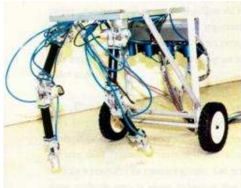
Figure 3.12: The photo (from [12]) shows the hybrid wheeled and legged robot SAP with dimensions 0.5 \times 0.3 \times 0.6 metres (L \times W \times H) . The wheels are passive and the system is used to test leg reference trajectories and control.
