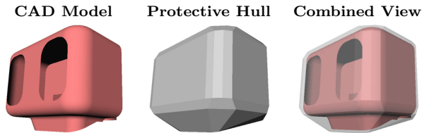
Figure 3: Protective Convex Hull for the head link.
