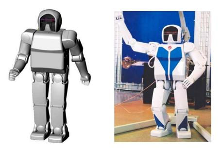
Fig. 1. SolidWorks model and photo of ARNE-02
