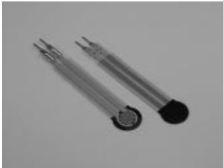
(c) Force sensor (FSR)
