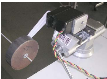
Fig. 2. Experimental evaluation of the actuator's response using a HITEC HS805BB servomotor
