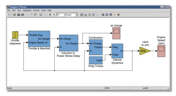
Simulink Control Design lets you perform linear analysis of nonlinear Simulink models.
