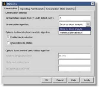
Simulink Control Design gives you control over the linearization algorithm.
