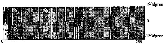
Figure 11: Sensory-behavior space. Vertical dots; a case of vision bumper pattern (256). Horizontal dot; safe direction to move (5 degrees/dot). Black; not safe to move, White; safe to move. Gray; no data.
