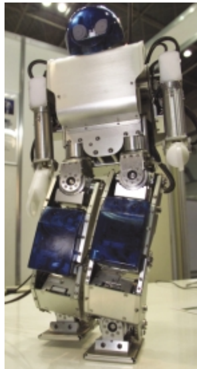
Fujitsu's HOAP-1 ambles along, relying on 20 motors and microcontrollers and an Intel MMX Pentium chip.
