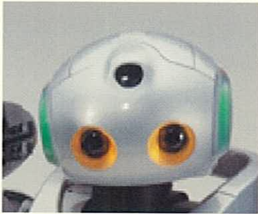
Fig.8 Vision sensor system inside the head
