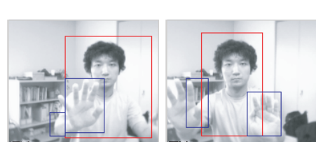
Fig. 3. A set of moving-regions obtained by QRIO's stereo cameras: They are clustered by disparity (distance) information.
