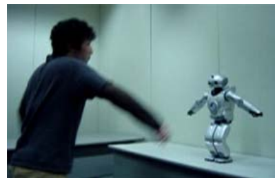
Fig. 4. Interactive dance application with QRIO: It reacts to the partner human's movement so as to follow its global rhythm and shape.
