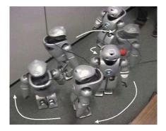
Fig. 15. Manuvoring experiment using combination of CPG and statemachine controller
