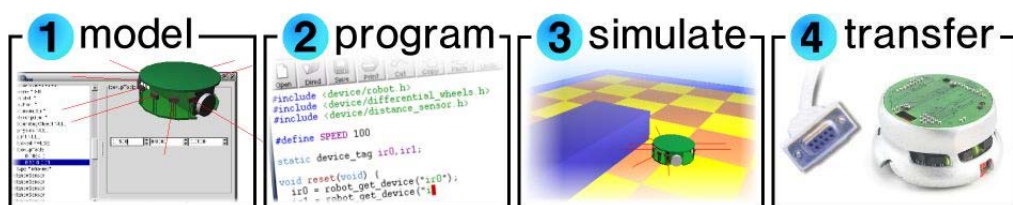
Figure 3.1: Webots development cycle of robot simulation.
