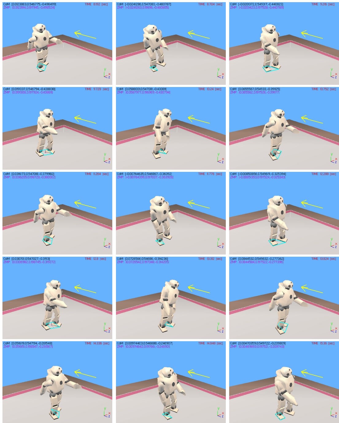
Figure 5.17: Snapshots of the external disturbance experiment. Compensation is done only using torso joints. The yellow arrow represents the external force acting on the robot (-0.2 [N]). (Continued).
