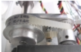
Fig. 2. Transmission belt with an adjustable tensile roller
