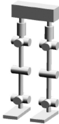
Figure 1: Diagram showing DOFs/joints of robot. Each cylinder represents one joint. In total, there are 12 joints - 3 at each hip, 1 at each knee, and 2 at each ankle.
