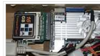
A 16-GB CompactFlash card installed in a 2.5" IDE port with adaptor
