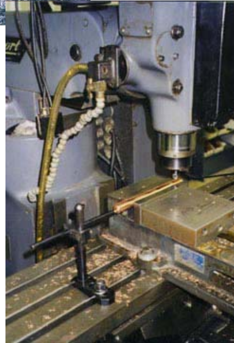
EMC retrofit on Bridgeport knee mill drilling copper tubing for heat exchangers at Flat Plate, Inc., York, PA
