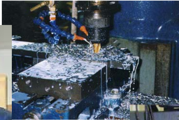
EMC retrofit on Wells-Index knee mill machining cast iron molds at Unique Machining, Millersville, MD
