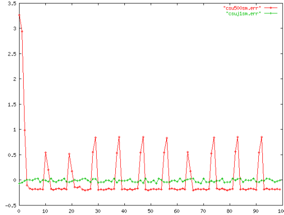
Figure 6. A comparison of uncompensated and compensated task jitter, with values 3.60 microseconds and 0.098 microseconds, respectively.
